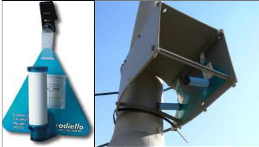
Figure 4: Passive sampling equipment
