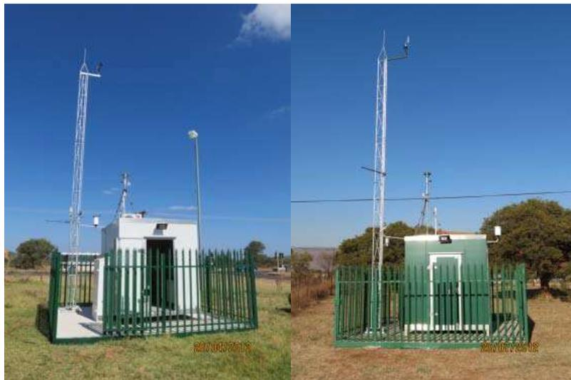
Figure 3: Examples of continuous ambient air quality monitoring stations
