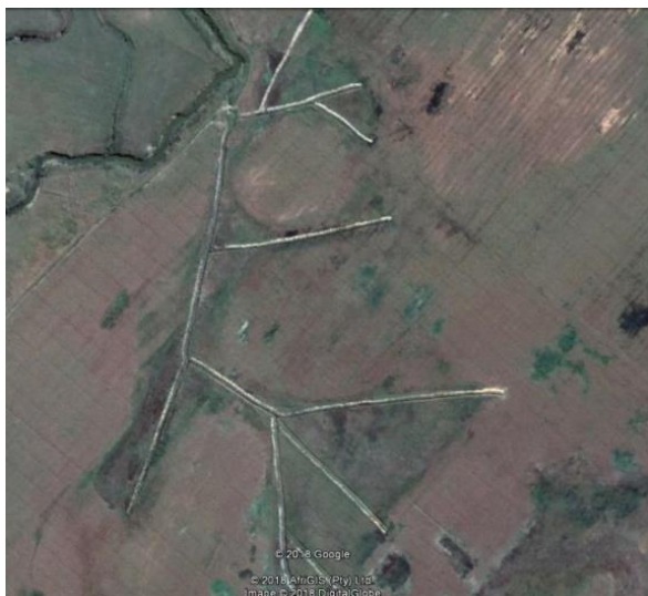
Figure 53: Series of drains draining a wetland for agricultural purposes.
